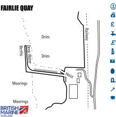
Fairlie Quay is starting the development process to become a full service marina and leisure craft service centre, and currently boasts the largest marine hoist on the Clyde with lifting capacity of 80 tons.
