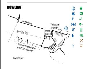
This attractive, historic basin is at the western end of the Forth & Clyde Canal, where it meets the River Clyde. The sea lock and canal dimensions are: length 20.47m; beam 6.35m; depth 1.83m and air draft 3.00m. Access is at 2 hours either side of HW, or as advised.
